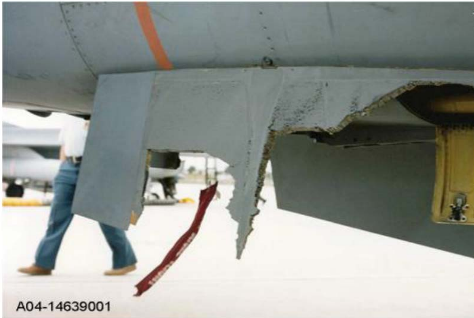
Figure 2. F-16 ventral fin damage on flight with LANTIRN
